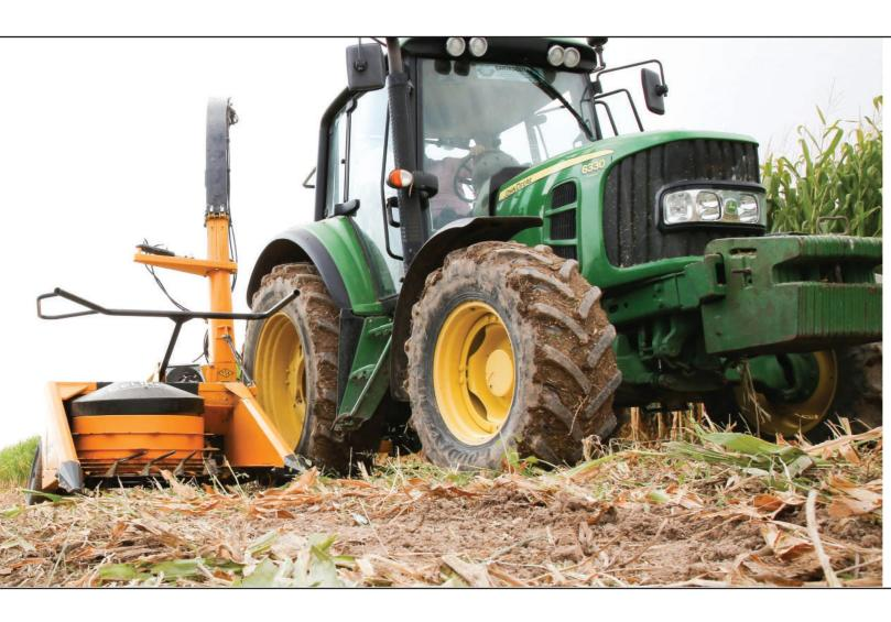
Row Independent Maize Chopper is designed specially to harvest various feed plants, forage and corn longer than 1 meter without considering any row in the field thanks to a wide harvester drum unit. The machine performs its task despite difficult harvesting conditions and removes opening row process problem that is seen
